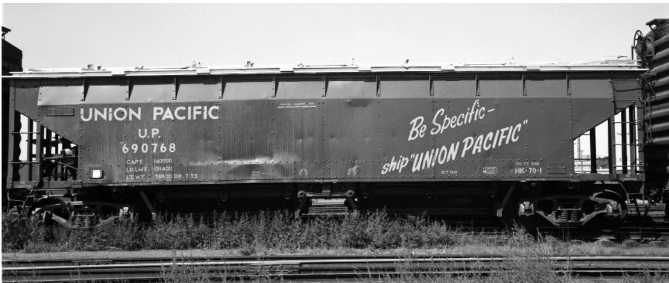
Union Pacific HK-70-1 690768 had the "6" added to its original car number when it received a roof for use in grain service. The UPHS recently placed an order with Atlas for a custom run of HO-scale HK-70-1 Hart ballast hoppers with anticipated delivery third quarter 2014. A resin casting of the grain roof is in development. – *Union Pacific Museum Collection*
